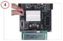
Vary the R56 potentiometer. The voltage is displayed with 12-bit resolution on the LCD module.
