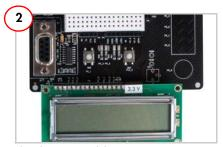
Plug the LCD module into port P8.
