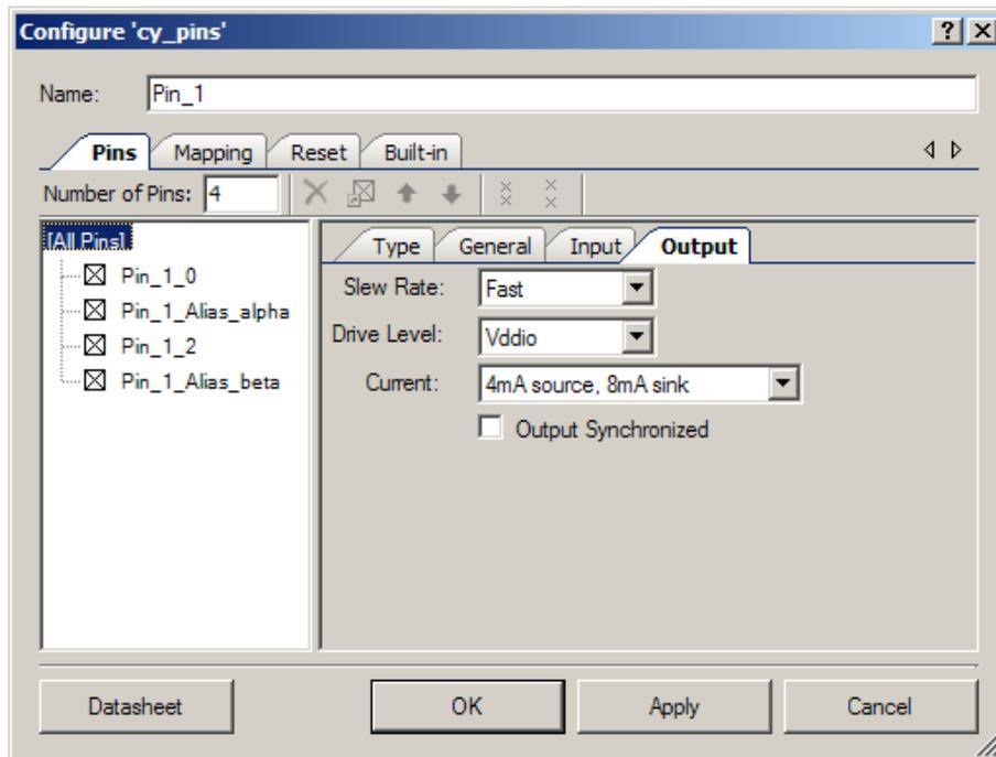
The **Output** subtab specifies output settings. If the pin type is not **Digital Output** or **Bidirectional** this tab is disabled because you do not need to specify output information.
