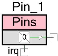
An Interrupt can be used in all configurations of the Pins component, as long as you include digital input.
