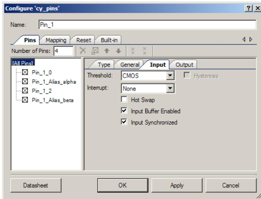
The **Input** subtab specifies input settings. If the pin type is not **Digital Input** or **Bidirectional** in the **Type** subtab, this subtab is disabled because you do not need to specify input information.
