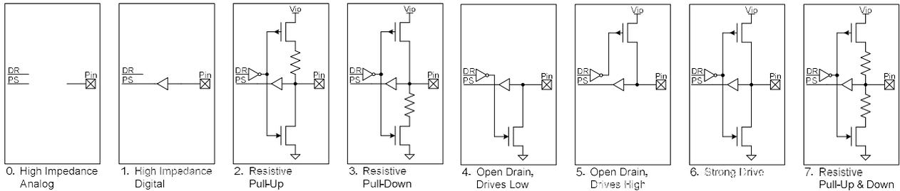
**Note** If any of the three resistive drive modes (**Resistive Pull Up**, **Resistive Pull Down**, **Resistive Pull Up/Down**) is used, setting the output drive level to **Vref** does not work.
