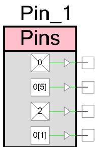
**Note** If the Pins component is set to **Display as Bus**, the display of the component does not display any locked pin assignments; however, the tooltip still displays this information.
