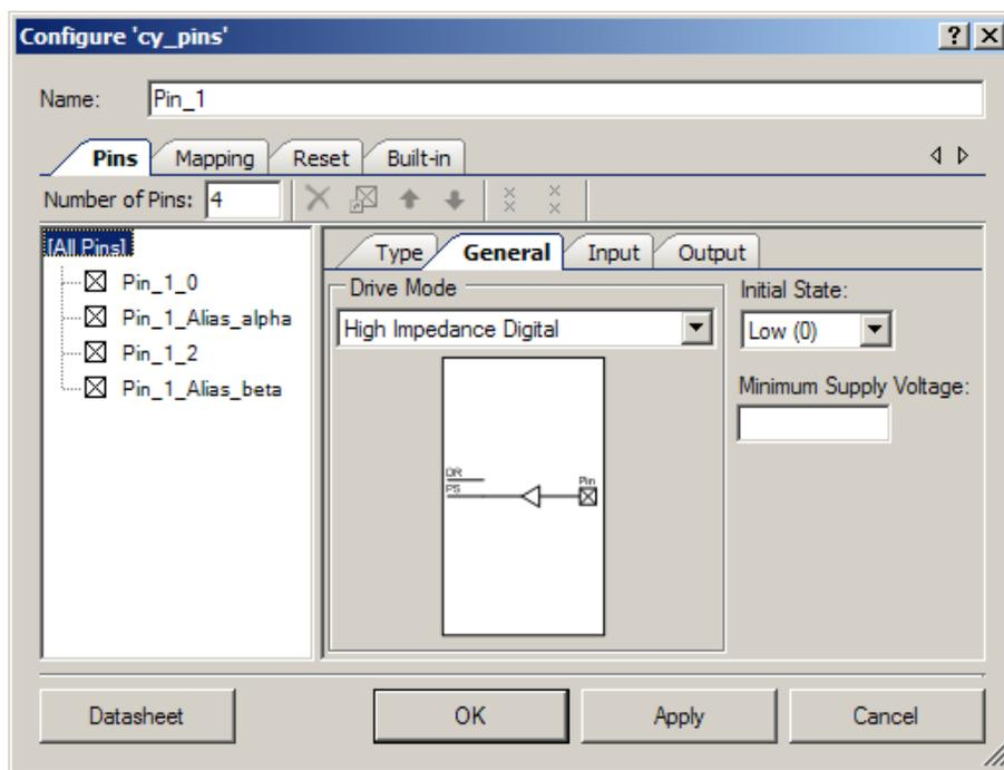
The **General** subtab allows you to set up parameters that apply to all pins, such as the drive mode, initial state, and minimum supply voltage of the selected pin. The settings on this subtab include:
